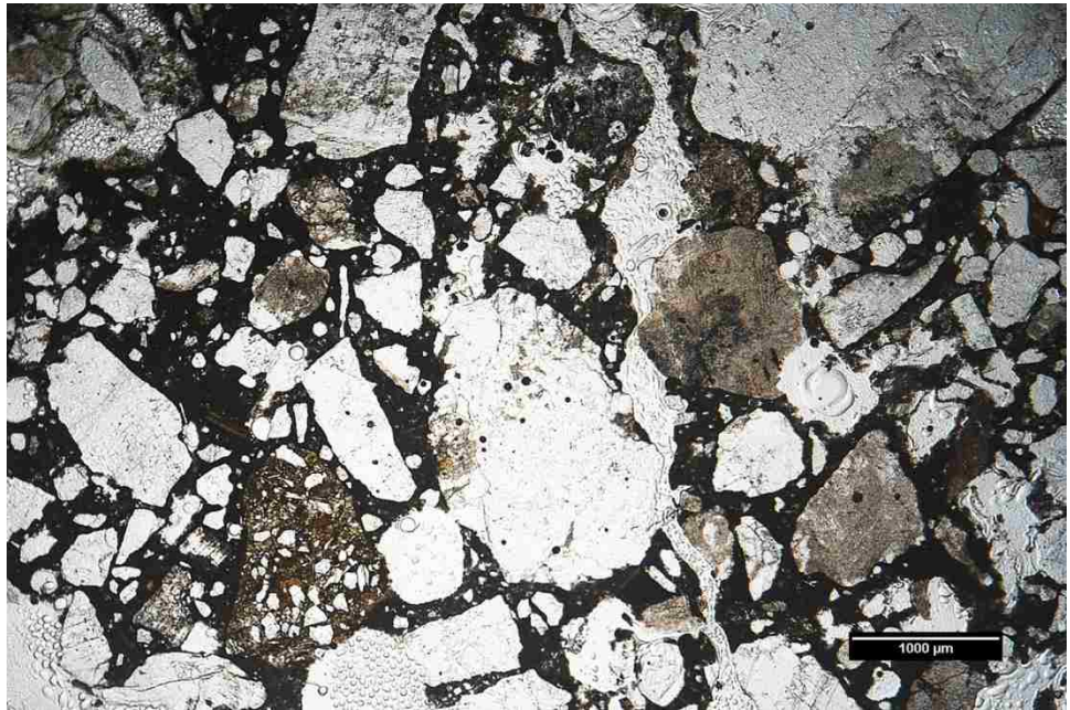
Figure 17. Aggregate with no signs of ASR (Source: DRP).
