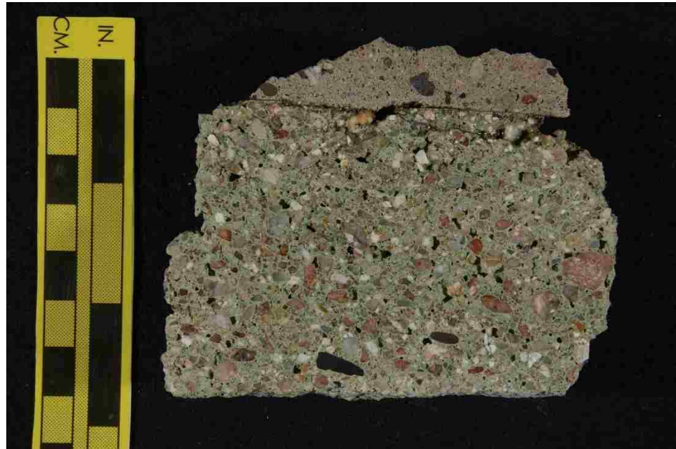
Figure 13 Sample polished and thin sliced for testing (Source: DRP).
