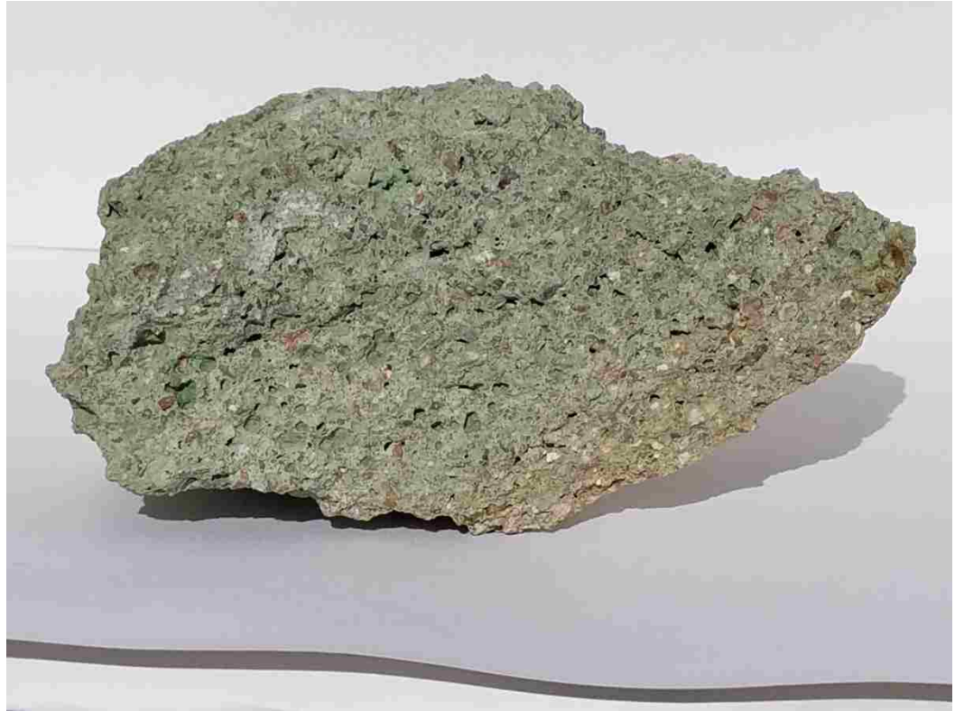
Figure 9. Sample of historic concrete from broken bench.
