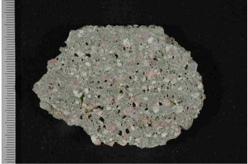
Figure 16. Phenolphthalein test, no staining (Source: DRP).
